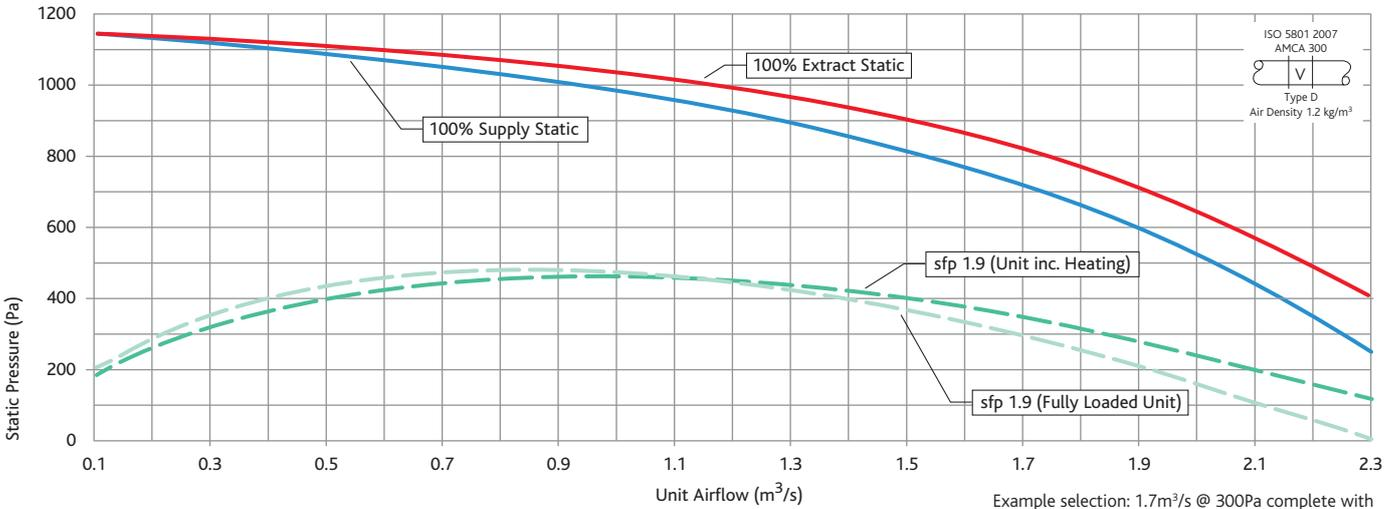
Example selection: 1.7m³/s @ 300Pa complete with LPHW heater, 2018 Thermal Wheel, LPHW frost coil, chilled water, attenuation and Ecosmart Connect control, SFP = 1.6 W(l/s).
