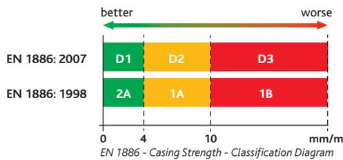
EN 1886 - Casing Strength - Classification Diagram
