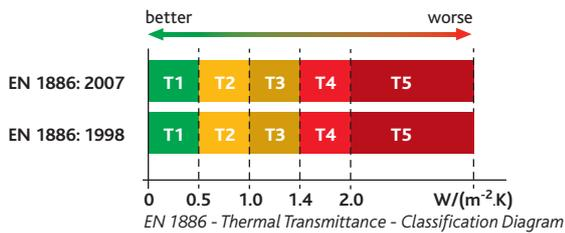
EN 1886 - Thermal Transmittance - Classification Diagram
