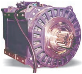
Traction Motor Type 6 FRA 6068 TM for 6000 HP Locomotive
