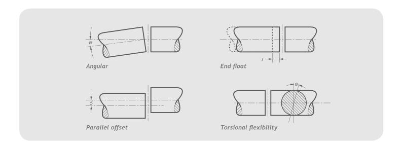
Flexible Couplings should be used to accommodate any combination of misalignment conditions described below.
