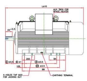
RINGED DIMENSIONS ARE AS PER IEC:60072-1 ALL DIMENSIONS ARE IN mm
