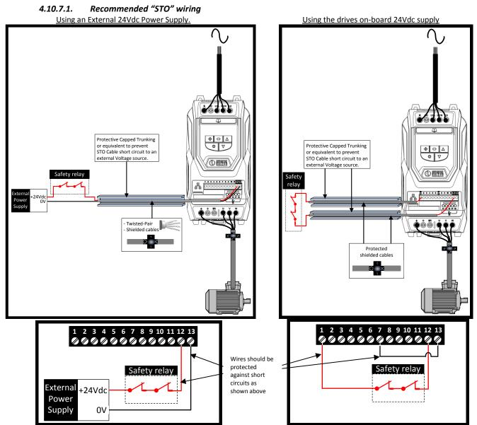
Note : The Maximum cable length from Voltage source to the drive terminals should not exceed 25 mtrs.
